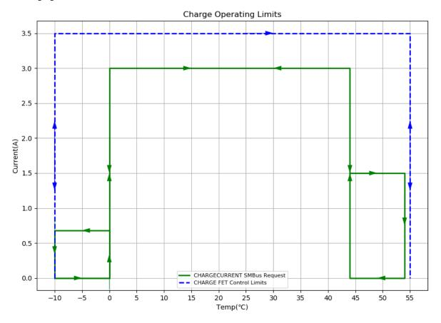
NOTE: If not charging & temperature > 45C then the battery enters Charge-Inhibit where ChargingCurrent() = 0 until temperature  $\leq$  44C.
