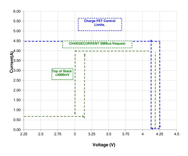
NOTE: The charging current requested from 3.0 to 4.2 V is defined by the temperature of the pack as shown in the preceding charge operating limits graph in this section. A 4.0A charge current is shown in this graph to represent the current defined by said graph.
