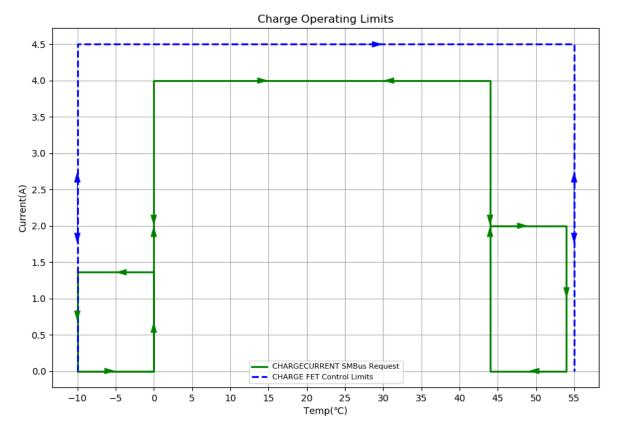
NOTE: If not charging & temperature > 45 °C then the battery enters Charge-Inhibit where ChargingCurrent() = 0 until temperature  $\le 44$  °C.
