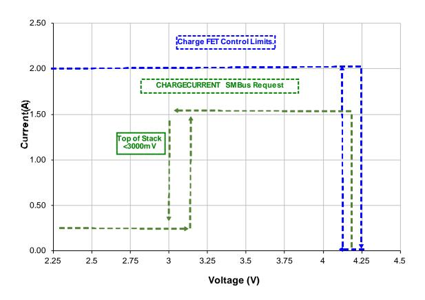
NOTE: The charging current requested from 3.0 to 4.2 V is defined by the temperature of the pack as shown in the preceding charge operating limits graph in this section. A 1.5A charge current is shown in this graph to represent the current defined by said graph.
